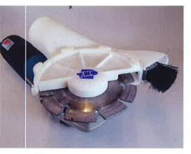
▲ To solve the problem of dust contamination during grinding, TNO Industrial Technology developed this direct vacuum system fitted to the equipment. Injection-moulding was prohibitive because only 10 were needed. Instead the SLS machine was used for their manufacture.
