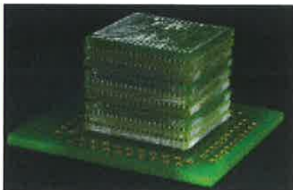
Footprint reduction using stacked microsystems.
