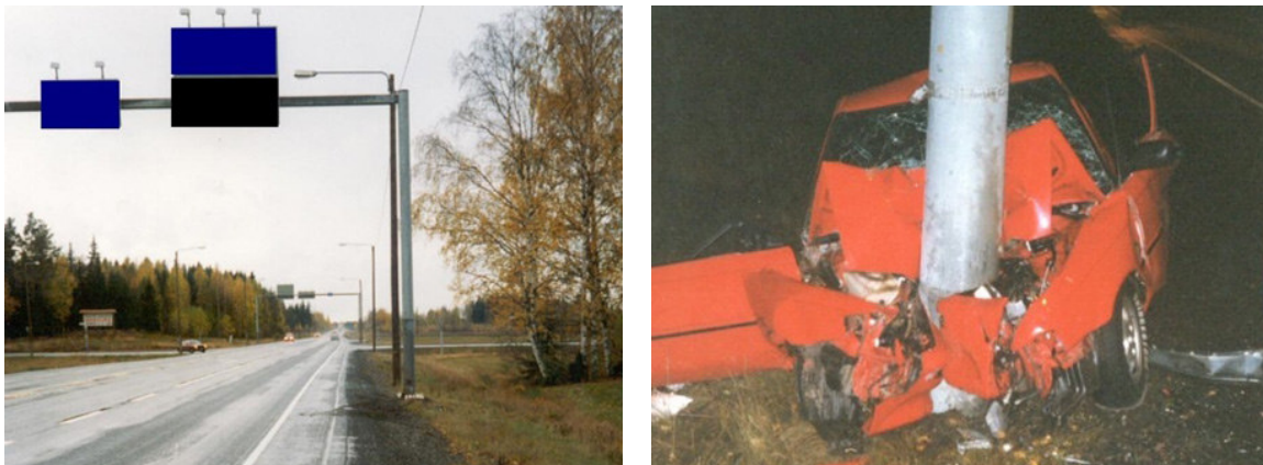
Figure 4.17. Unprotected gantry poles in the safety zone are fatal hazards (Photo, VALT)
