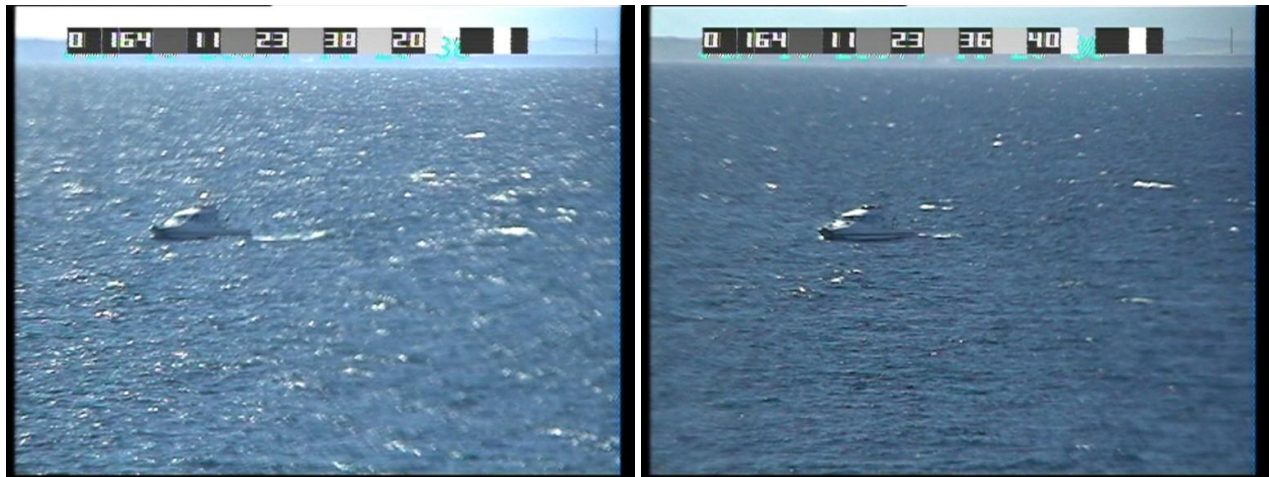
Figure 9: Visible light polarisation imagery of the small scientific work boat. Left horizontal, right vertical polarisation.
