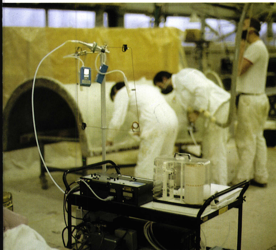
Measuring the concentration of styrene in the air exhaled by workers in the polystyrene industry.
