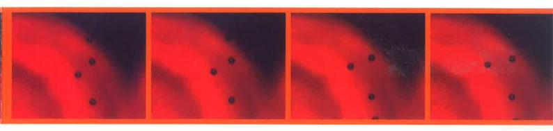
guided. The series of photos at the top of this page covers a timeline in which one in four droplets is diverted from the jet. The other unused droplets are captured and recirrulated.
