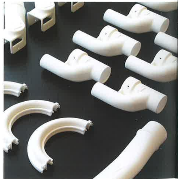
Using Selective Laser Sintering (SLS) and Fused Deposition Modelling (FDM) functional components are made for various hand tools with dust extraction.
