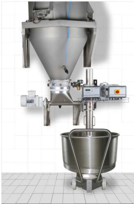
Picture 6: The flour-moistening machine (source: Reimelt)
