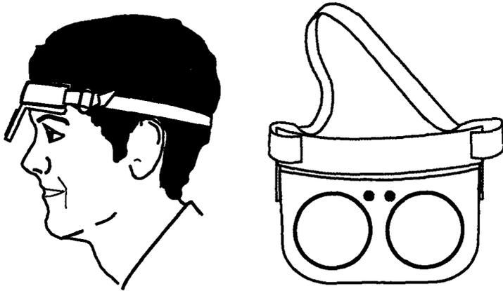
Figure 6.13 The dark glasses worn during oxy-gas cutting.
