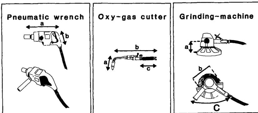
Figure 6.1 The pneumatic wrench, oxy-gas cutter, and grinding-machine, that were used in the experiments. Dimensions are presented in table 6.3.
