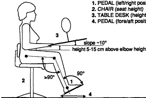
1. The PEDAL shall be positioned right in front of the operating foot, while its inclination shall be adjusted in such a way that the angle between the lower leg and the foot is about 90°.
