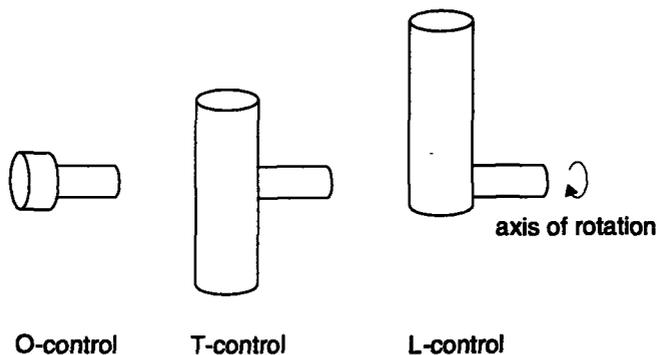
Figure 2.4 Schematic side view of three types of rotary controls. Reprinted from Van der Vaart (1995), with kind permission from Delft University Press.
