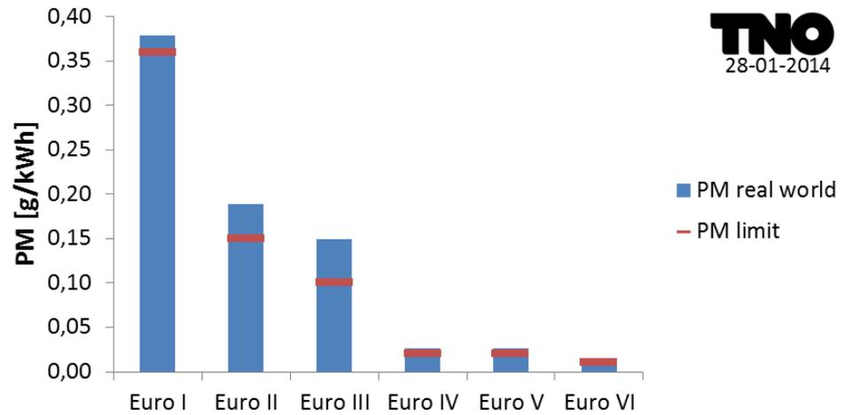
Figure 8: PM real world emissions and type approval limit values of heavy duty vehicles.
