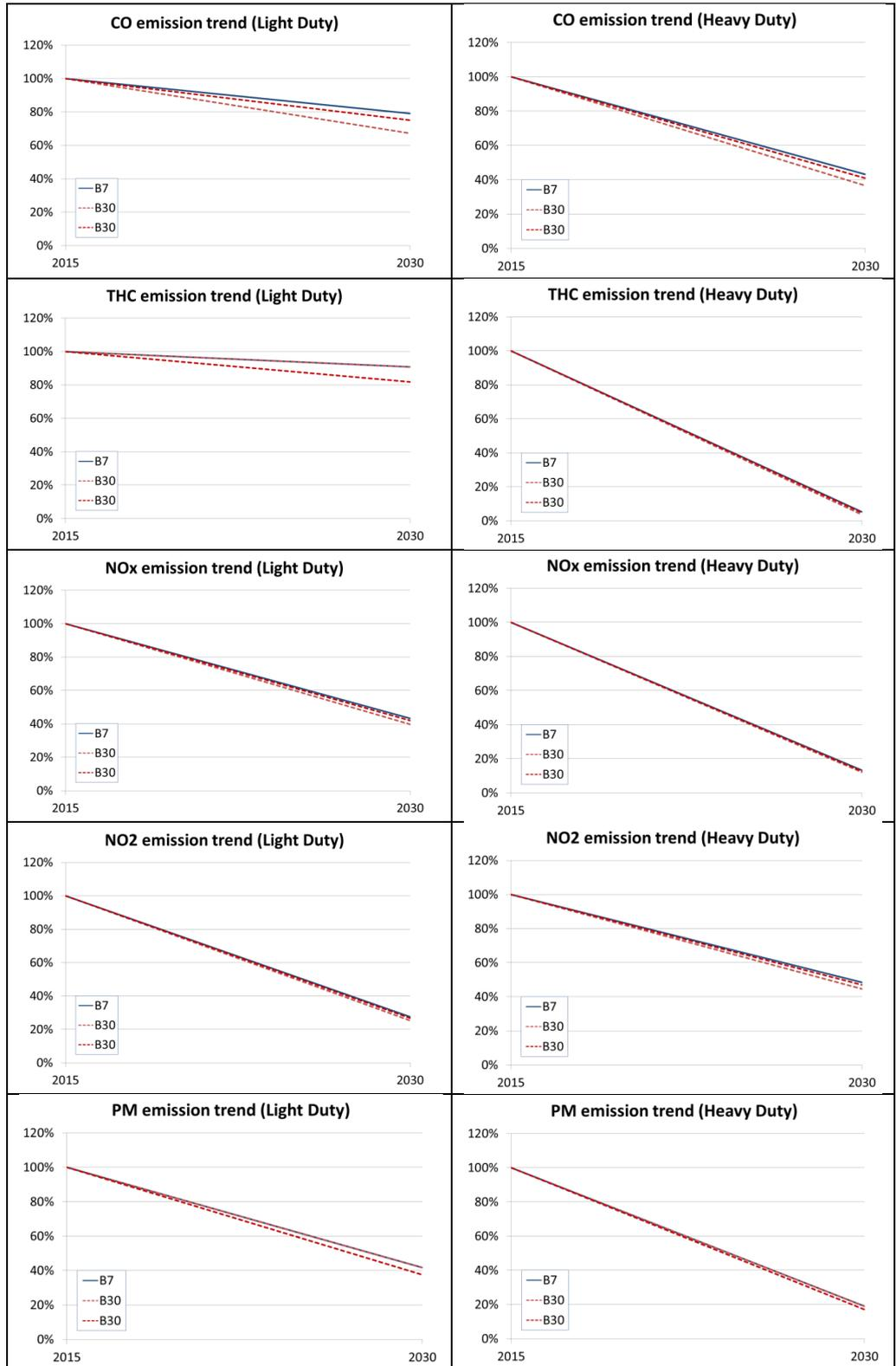
Figure 1: Predicted emissions trends 2015-2030 – Light Duty and Heavy Duty vehicles and the effects of increased biodiesel blends.
