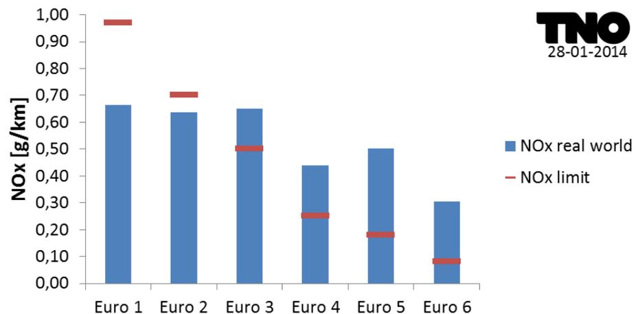
Figure 5: NOx emission factors and type approval limit values of diesel passenger cars.
