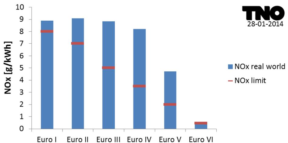
Figure 7: NOx real world emissions and type approval limit values of heavy duty vehicles.
