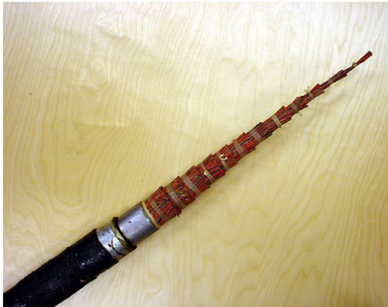
Figure 1: A typical cable in use in the Dutch copper access network. These cables contain many hundreds of individual wire pairs. Source: TNO
