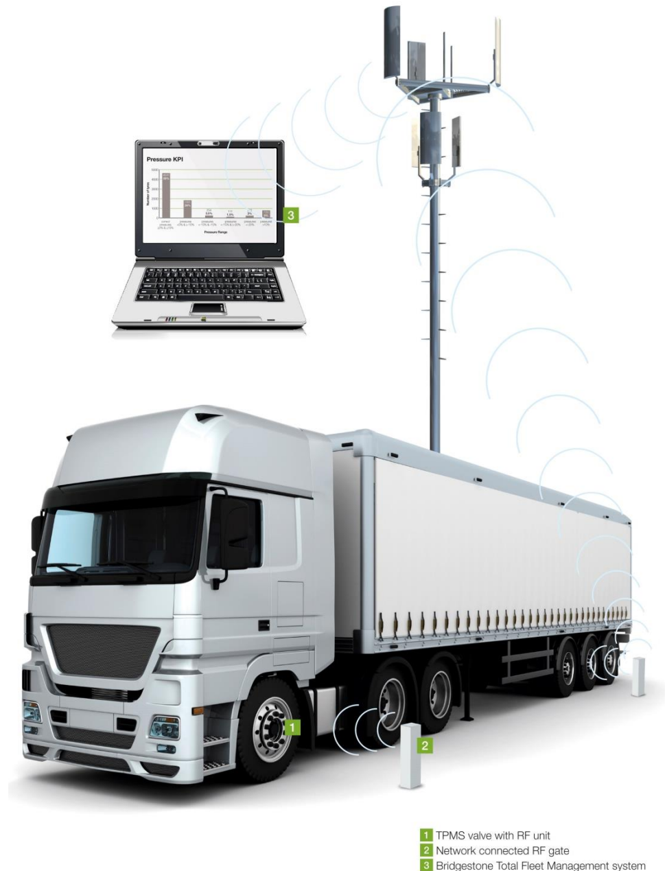
Figure 53: Bridgestone TPMS with Tyrematics [BS, 2013]
