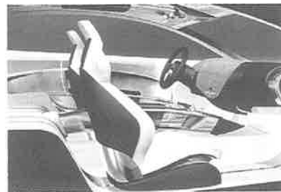
Figure 15.2 The Volvo Safety Concept Car makes adjustments to the interior based on the eye position of the driver
