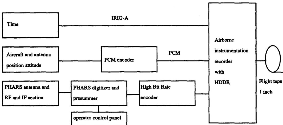
Figure 2. Block diagram of the PHARS airborne system.
