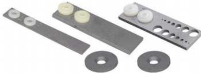
Figure 6-1. Example of corrosion coupons(“Rohrback Cosasco Systems,” n.d.)
