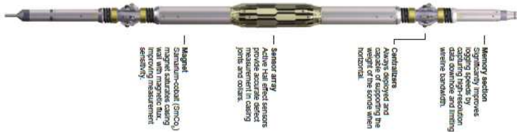
Figure 6-4. Example of a magnetic flux leakage tool(Weatherford, 2010b).
