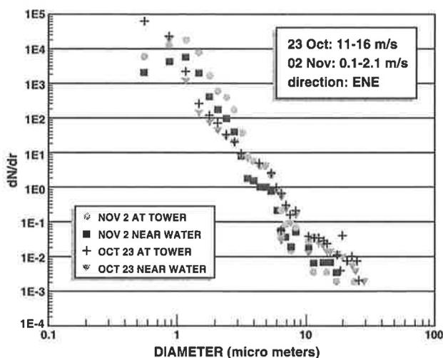
Figure 4. Measured aerosol-size-distributions at MPN.
