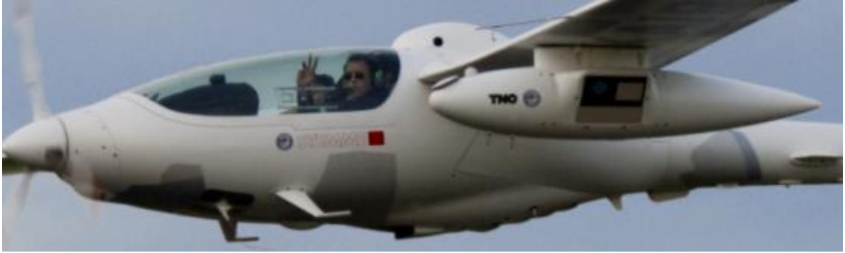
Figure 8. Small airplane used for the SAR imaging tests. A pod was mounted below the left wing. DriftLess was placed in the front of the pod
