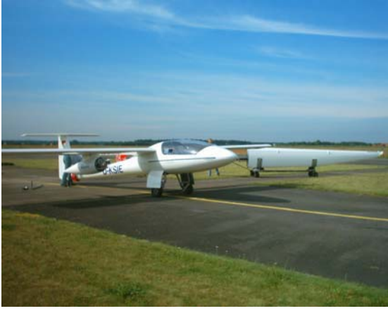
Fig. 1. The Stemme motor glider, the pod is attached under the right wing. In the back the wing tips are visible. The tips can be taken off to accommodate transportation of the glider.
