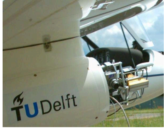
Fig. 2. The FM-CW SAR demonstrator system installed in the pod. In front of the pod the digital camera, the FM-CW front end and the GPS receiver are clearly visible (from left to right).
