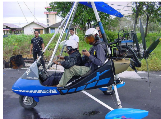
Fig. 1 Ultralight aircraft used as platform for the radar
