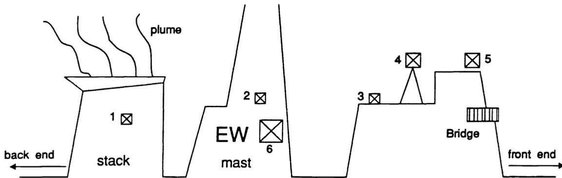
1 = port and SB thermocouple; 2 = port and SB radiometer and thermocouple, 3 = deck radiometer and thermocouple, 4 = double radiometer, 5 = weather station + GPS antenna, 6 = "radarhut" with 2 PC's and data acquisition.
