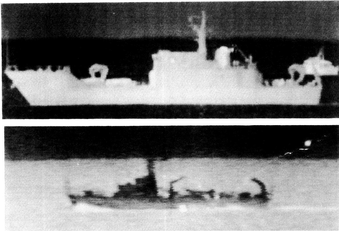
Fig. 1. IR imagery of ship in Livorno during SIVEX trials, showing contrast inversion from one day to next day due to drop in air temperature.
