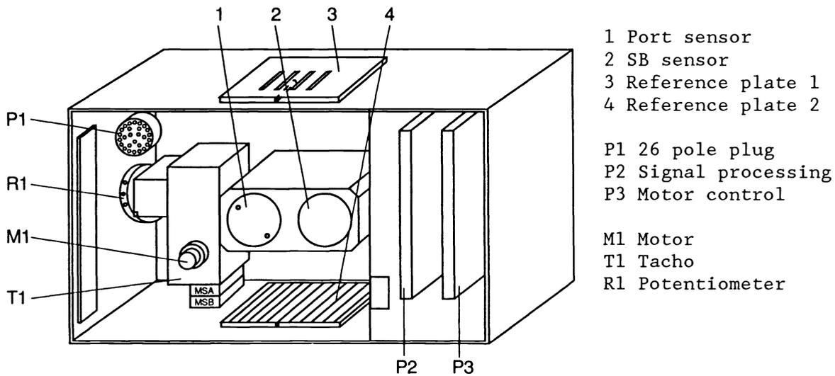
Fig. 3 Schematic view of double radiometer
