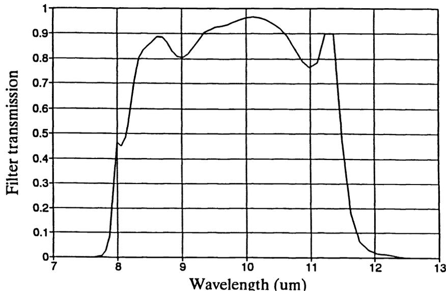
Fig. 4 Filter transmission for radiometers.
