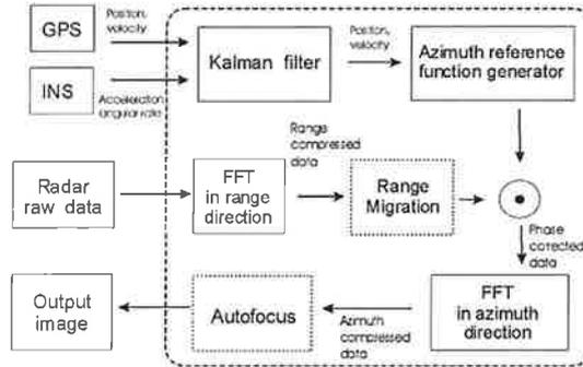
**Figure 3.** Basic logical flow diagram of the SAR processor to be applied. GPS and INS input data are used to reconstruct the actual flight path. Raw data are processed with FFT's in range and in azimuth direction to get the output image. Dotted blocks will be the object of near future work.
