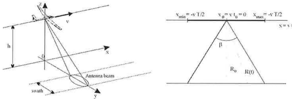
**Figure 1.** Geometry of the SAR system. The point target is in the antenna beam as long as  $x$ -coordinate of the antenna position is within the interval  $(x_{min}, x_{max})$ .  $\beta$  is azimuth beamwidth of the physical antenna.
