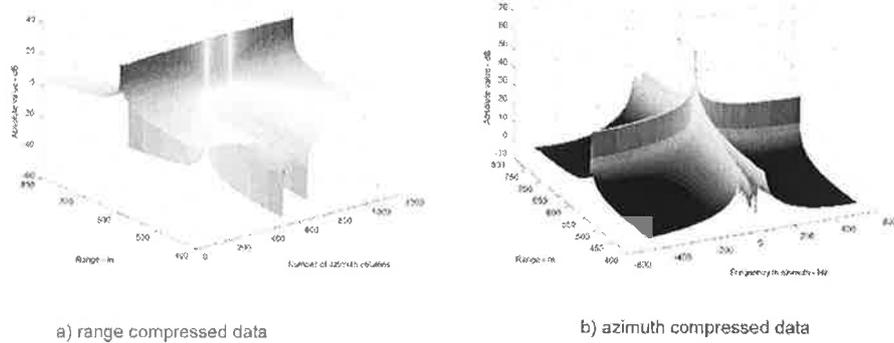
Figure 4. Simulation results of a single target at a nominal range of 600 m and processing 1024 sweeps are reported. In a) it is shown the range compressed data while b) illustrates the response after phase correction and azimuth compression.
