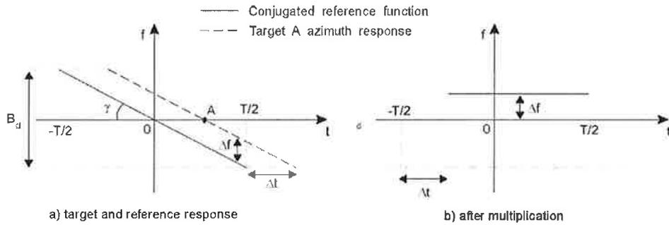
**Figure 2.** a) The target A is displaced of  $\Delta x = v\Delta t$  with respect to the origin where the azimuth reference function is centered and it illustrates how  $\Delta t$  is proportional to  $\Delta f$ ; b) after multiplication the frequency is constant and equal to  $\Delta f$  in the shadowed area, that is the time the target A is in the antenna beamwidth centered in zero.
