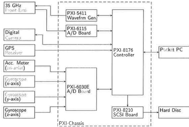
Fig. 3: The block diagram of the FM CW SAR demonstrator system.
