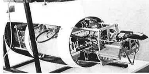
Fig. 2: The FM-CW SAR demonstrator system installed in the standard pod.
