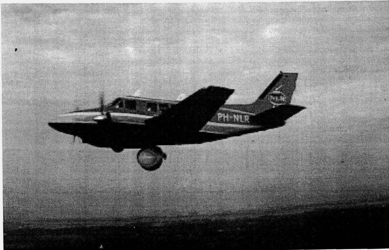
Figure 2. DUTSCAT system mounted under the Queen Air airplane
