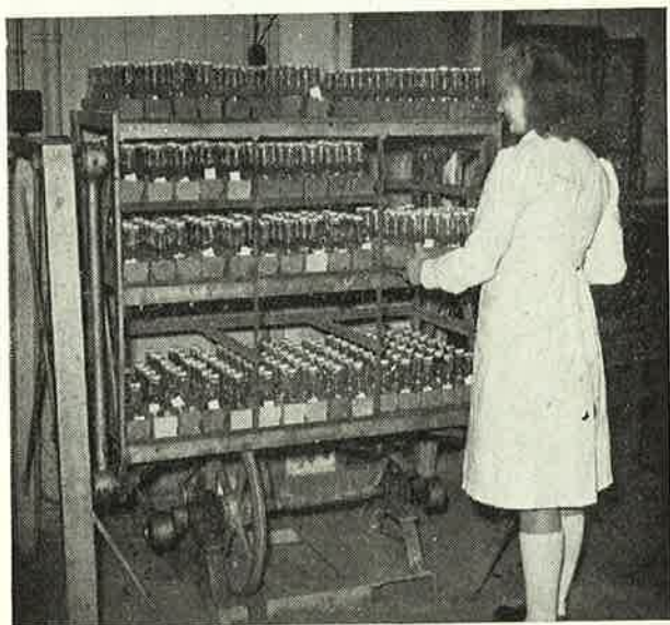
Vibrating machine used to extract soil for measurement of phosphate and potash content.
