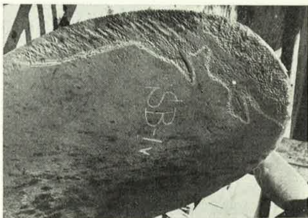
Cavitation and erosion of a ship's propeller.
