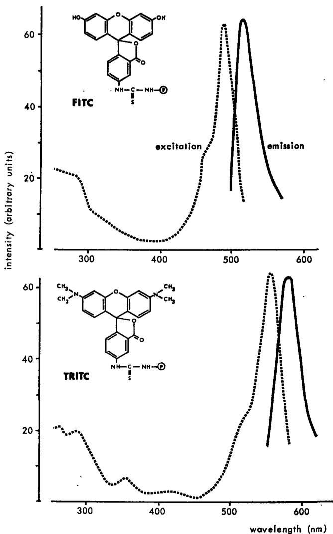
Figure I-1. Structural formula, excitation and emission spectra (redrawn from Hansen, 1964) of the two most commonly used fluorochromes in immunofluorescence microscopy: fluorescein isothiocyanate (FITC; molecular weight 379.39) and tetramethyl rhodamine isothiocyanate (TRITC; molecular weight 431.13). In the formula, P stands for protein.
