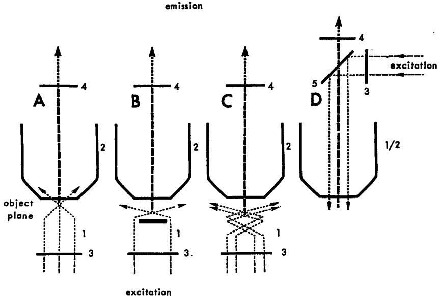
Figure I-2. Schematic representation of different illumination systems in immunofluorescence microscopes.
