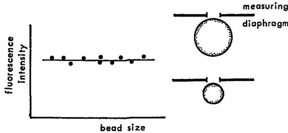
Fluorescence intensity of individual beads (●) is independent of bead size
