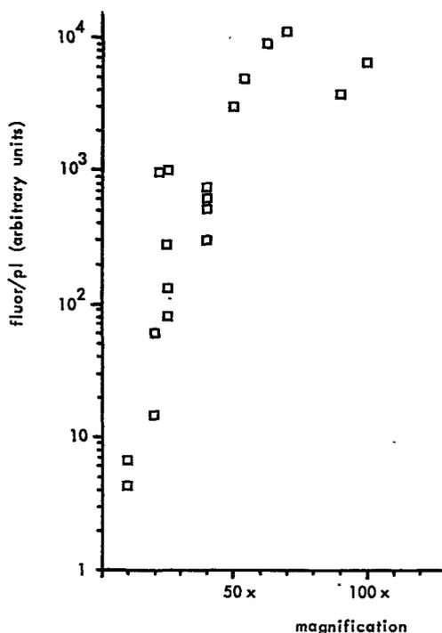
Figure II-5. The influence of the magnification of objectives on the fluorescence per picolitre of aminoethyl-Sephadex beads stained with FITC. Fluorescence and diameter of individual beads were measured. Each value represents the average of 15 individual bead measurements. The light source (CS 100 W) and collector lens were adjusted for each objective in order to fill the back entrance pupil of the objectives optimally. Eyepiece:  $6.3\times$ .
