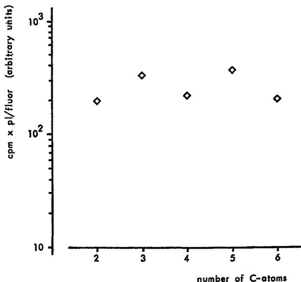
Figure III-2. The influence of spacers on the fluorescence of FITC. Sepharose beads were activated with cyanogen bromide. The activated Sepharose was reacted with 0.5 M diaminoethane, diaminopropane, diaminobutane, diaminopentane and diaminohexane. These beads were reacted subsequently with FITC-<sup>14</sup>C after deactivation of the residual active groups with ethanolamine. Fluorescence per picolitre and the radioactivity of the different bead species were measured.
