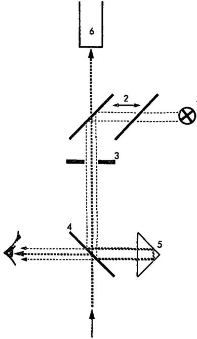
Figure VI-3. Construction of an automated microfluorometer.
