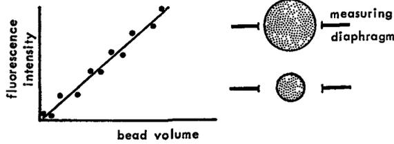
Fluorescence intensity of individual beads (●) is directly proportional to the volume of the beads
