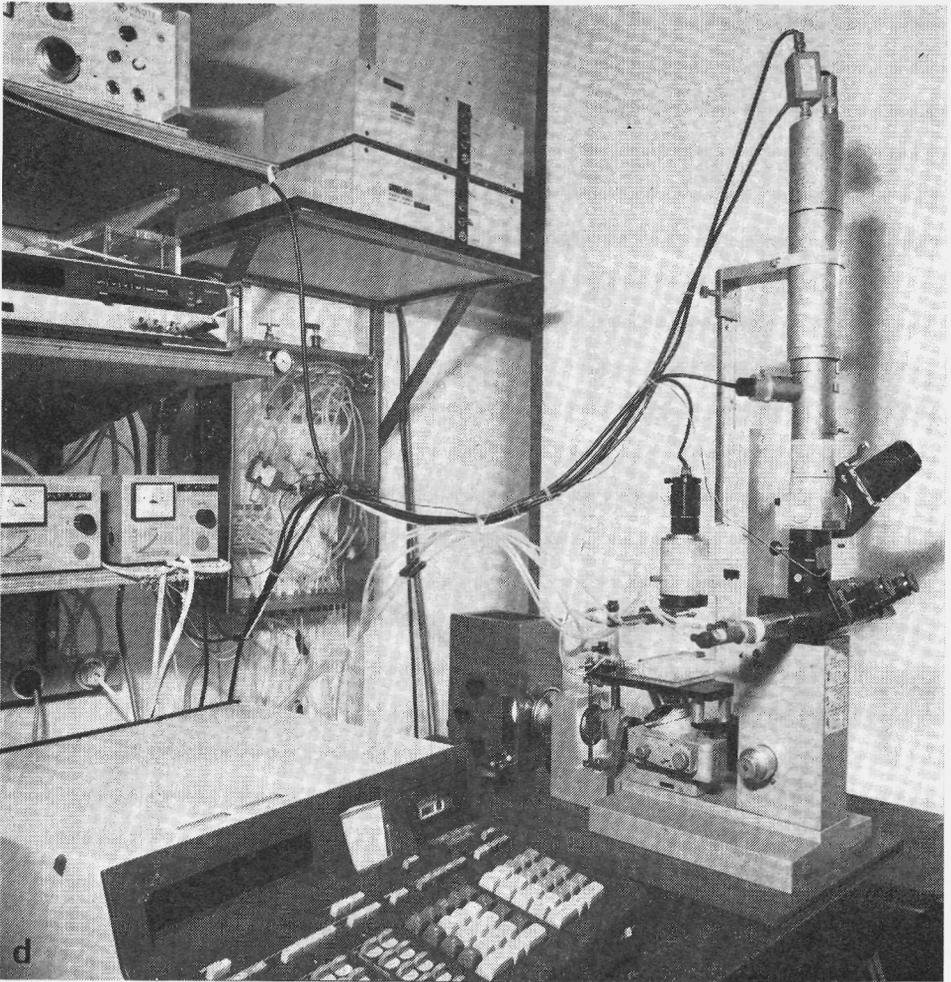
Figure VI-2d. General view of the automated Leitz Diavert inverted microfluorometer.
