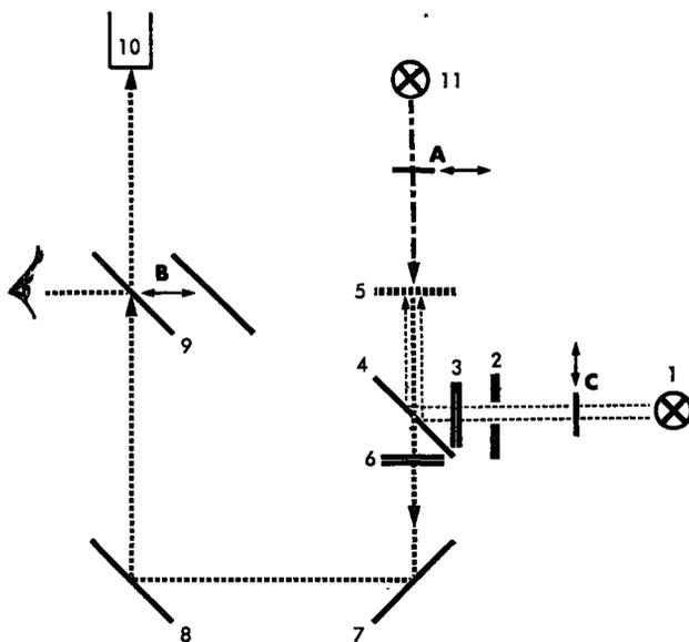
Figure VI-1. Schematic representation of the optical pathways in the Leitz Diavert inverted microscope equipped for epiillumination and fluorometry.
