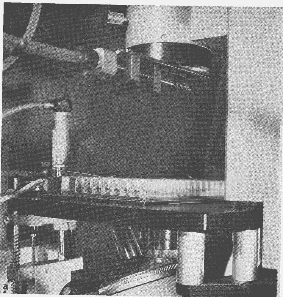
Figure VI-2a. Construction of an automated microfluorometer. Construction of shutter A (see Fig. VI-1) in the diillumination pathway. The cylinder is a DG-6-40 (Festo-Maschinenfabrik G. Stoll).
