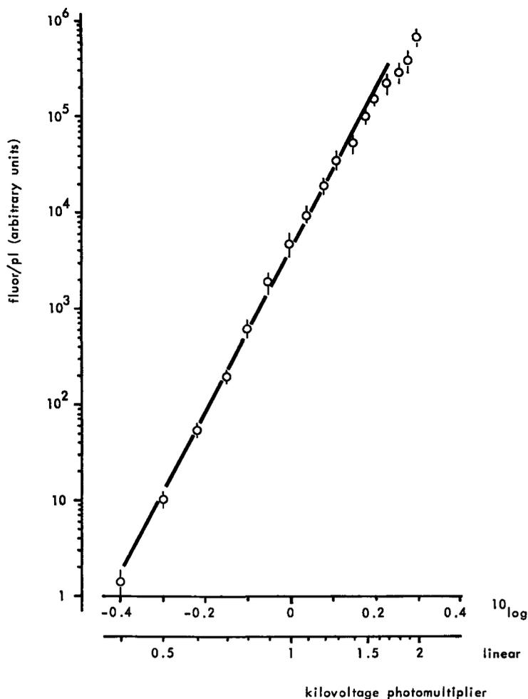
Figure II-2. The influence of photomultiplier voltage level on the fluorescence per picolitre of amino-ethyl-Sephadex beads stained with TRITC. Fluorescence and diameter of individual beads were measured. Each point represents the average fluorescence/picolitre value of 15 individual beads. Bars indicate standard deviations. Objective:  $25\times/0.60\text{ W}$ ; eyepiece:  $6.3\times$ .
