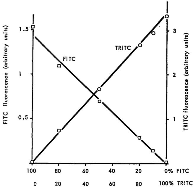
Figure V-11. Test for the interference with FITC emission by TRITC in aqueous solutions. Solutions of 0.1 mg/ml TRITC and 0.1 mg/ml FITC in 0.05 M carbonate buffer pH 9.5 were mixed in different proportions. The fluorescence of FITC and TRITC was measured in a microcuvette using a  $3.2 \times /0.07$  objective.
