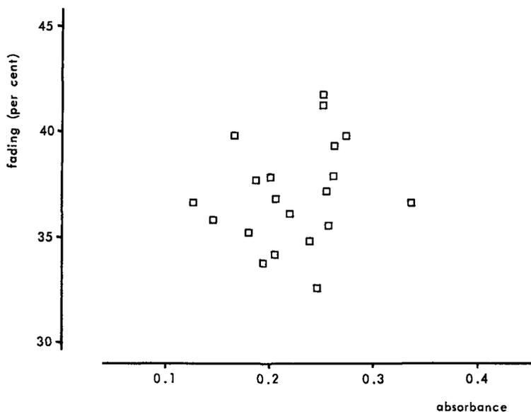
Figure III-4. Fading of FITC bound to aminoethyl-Sephadex beads. The degree of fading and the absorbance of individual beads were measured. The fading is expressed as the percentage of the initial fluorescence value remaining after 20 consecutive measurements (taking 120 seconds). The absorbance of individual beads was measured as described by Haaijman and van Dalen (1974). The absorbance is directly proportional to the amount of FITC present on the beads.
