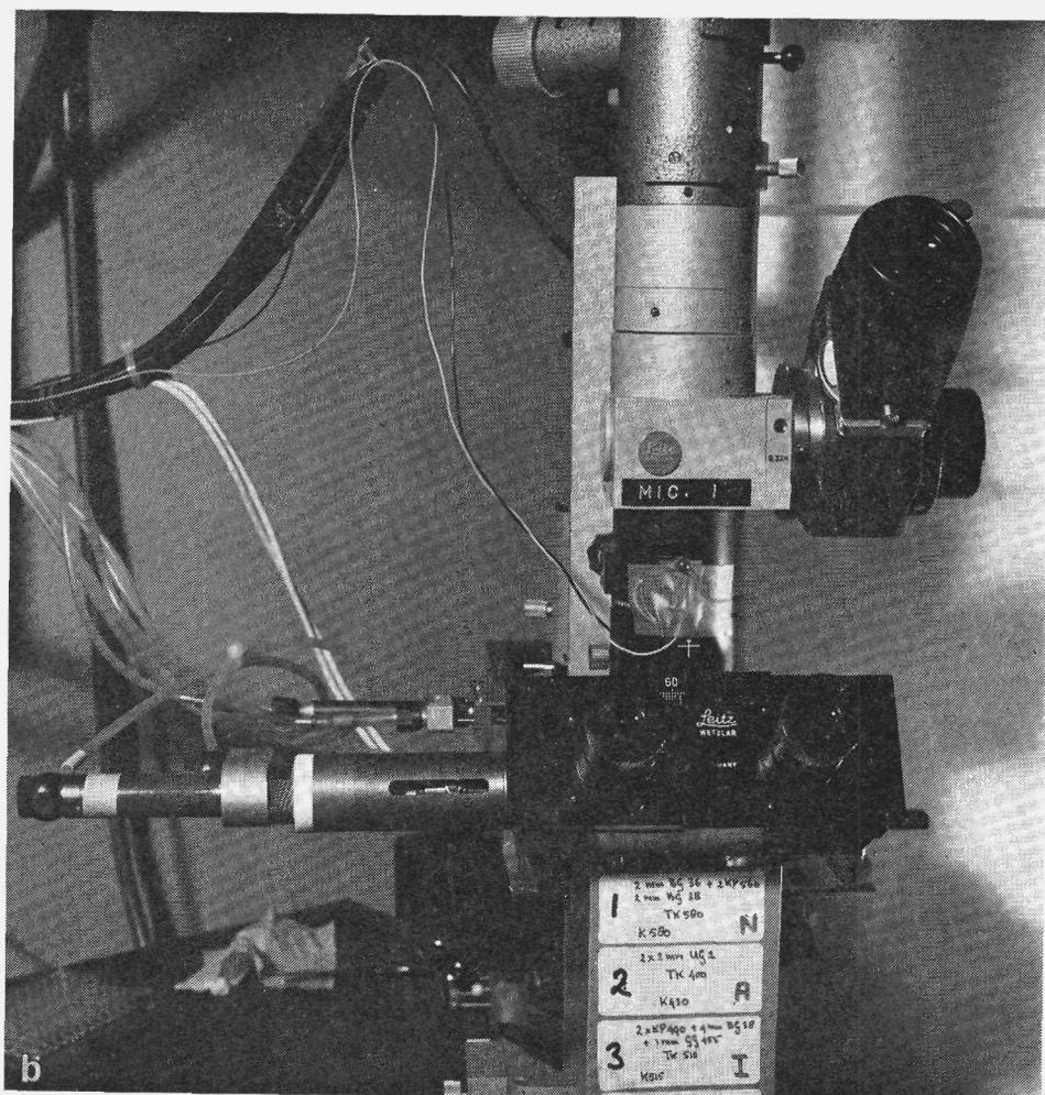
Figure VI-2b. Construction of shutter B (see Fig. VI-1) for the photomultiplier. The prism in the binoculars is moved with a DG-12-25 cylinder.
