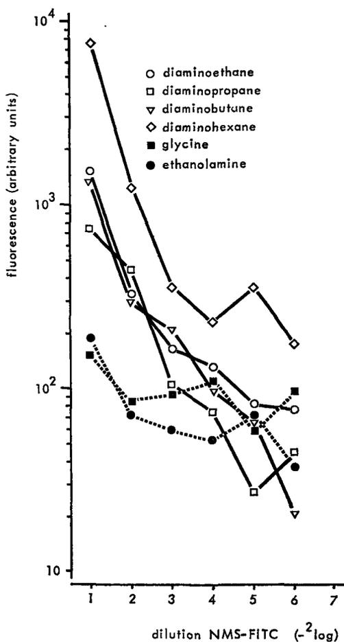
Figure IV-3. Influence of different deactivators on the nonspecific reaction. Sepharose beads were activated with cyanogen bromide. Activated beads were incubated with 0.5 M of the indicated compounds for 8 hr. The beads were incubated subsequently with different dilutions of a FITC conjugated normal mouse serum (NMS-FITC) in order to estimate the degree of nonspecific adherence with the different bead species. Each point is the average fluorescence intensity of at least 5 individual beads.
