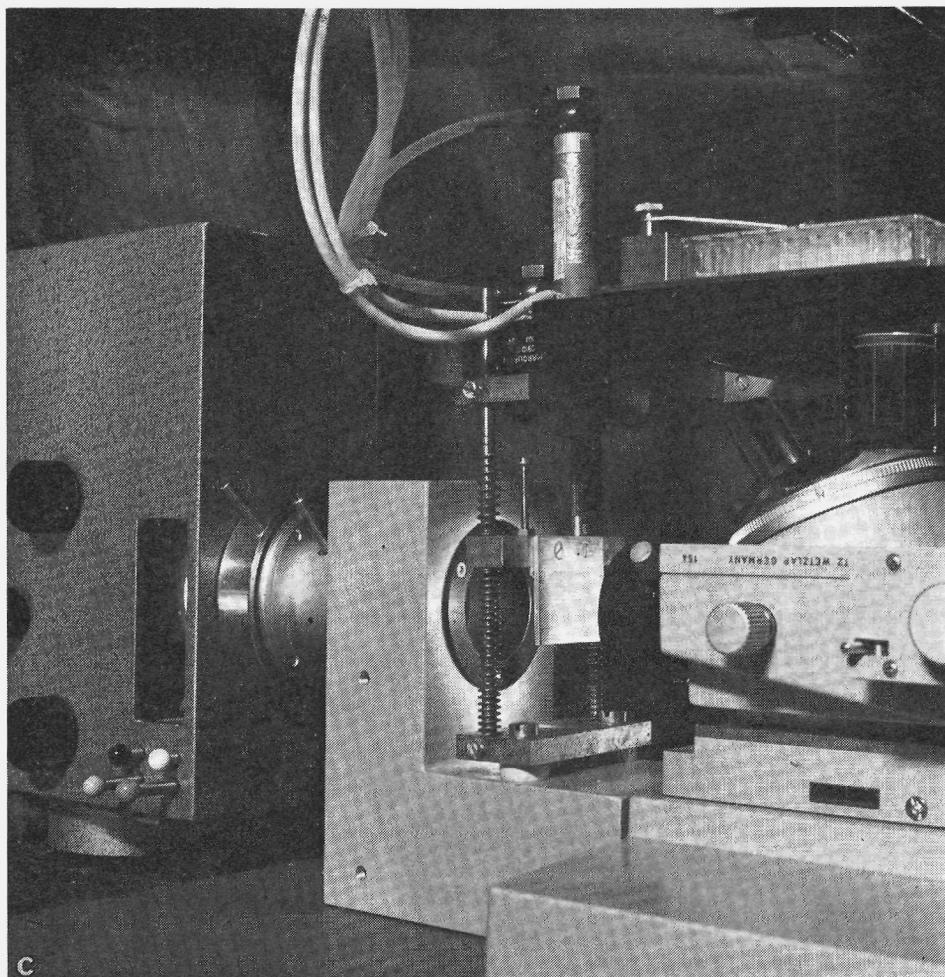
Figure VI-2c. Construction of shutter C (see Fig. VI-1) in the excitation pathway. The cylinder is a DG-12-25. The adjustable screw on the shutter blade presses against the microswitch if the shutter is fully opened.
