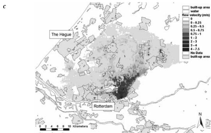
Figure 2: Case study: flood characteristics computed with the 2D hydraulic model: (a) time of inundation (hours after failure of the river dike), (b) maximum water depth (m), (c) maximum flow velocity (m/s)
