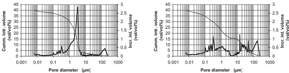
Figure 9: Two plasters with identical porosity values, but completely different built up of their pore size distributions. Left: A gypsum-lime plaster with water repellent; right: Weber et Broutin Terrassane render (N.B. Neither of the examples are from the COMPASS-evaluation test described here.)
