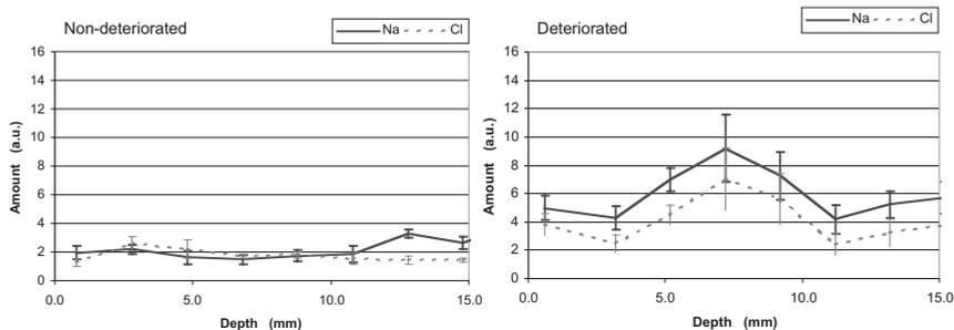
Figure 3: Salt profiles as found in Terrassane render. Left non-deteriorated sample; right deteriorated sample. Error bars indicate variation based on five parallel line measurements.
