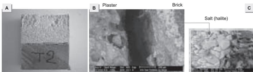
Figure 12: Final result after COMPASS-TEST for a trass lime Tubag plaster with a mass water repellent. Macroscopic view (a). ESEM observations: plaster/brick interface (b), detail of salt crystals (c).
