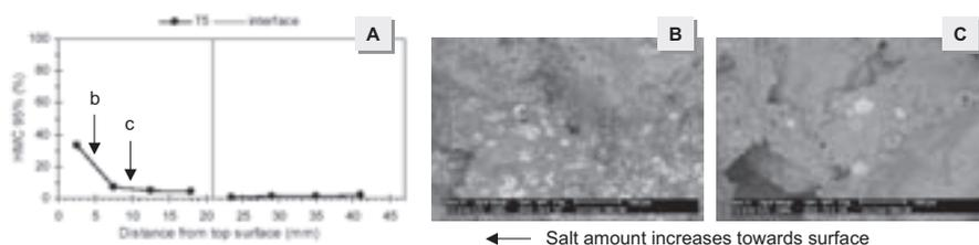
Figure 13: Distribution of salt (halite) over the plaster thickness as determined by HMC (a) and observations by ESEM (b and c). The locations of ESEM images are indicated in the HMC graph.
