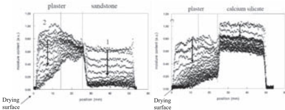
Figure 8: Results of drying experiments in NMR setup: plaster on Bentheim sandstone (left), plaster on calcium silicate stone (right) [Petković, 2004].
