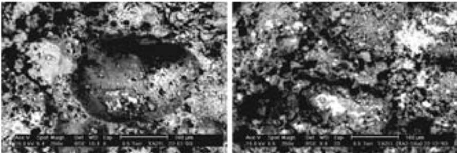
Figure 2: Increase in salt content going deeper into the render of the deteriorated sample. 10 mm depth (left), 15 mm depth (right).
