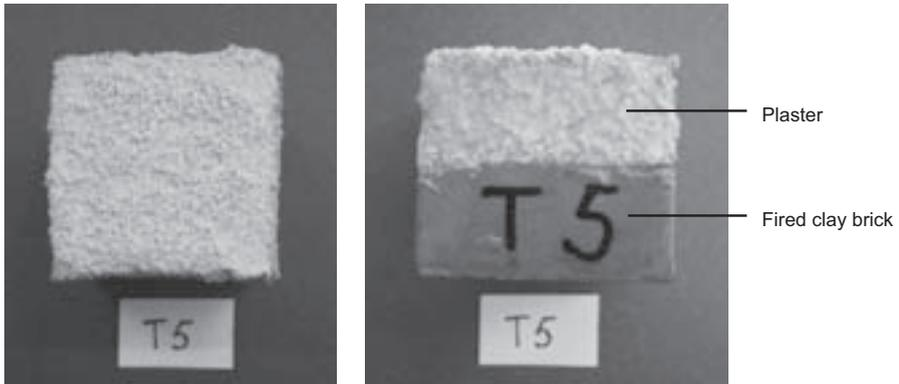
Figure 10: Final result after COMPASS-TEST for home made TNO plaster. View of topside (left), view of side (right).
