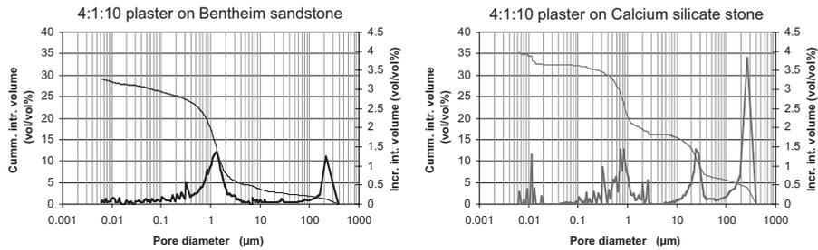
Figure 7: Pore size distributions from identical plasters applied on two different substrates: on Bentheim sandstone (left), on calcium silicate brick (right).
