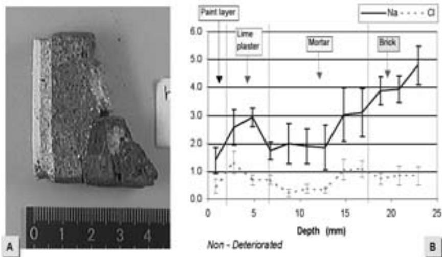
Figure 4: Cross-section of a non-deteriorated sample from Engelmundus church (a), with corresponding sodium and chloride profiles through the various layers (b).
