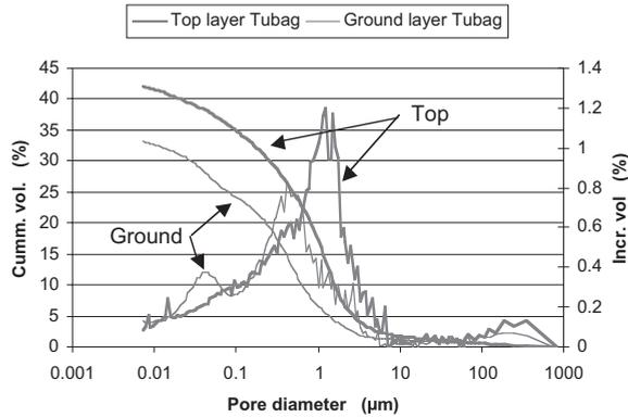
Figure 5: Pore size distribution of first and second plaster layer applied right after each other [Wijffels, 1996]. Tubag is a commercial name of a trass-lime based plaster with a mass water repellent.
