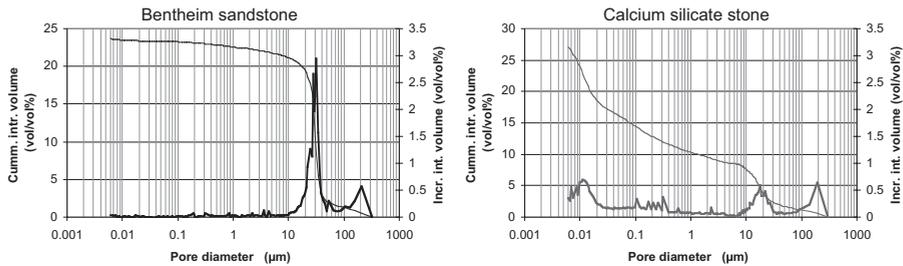
Figure 6: Pore size distributions of Bentheim sandstone (left) and a calcium silicate brick (right).
