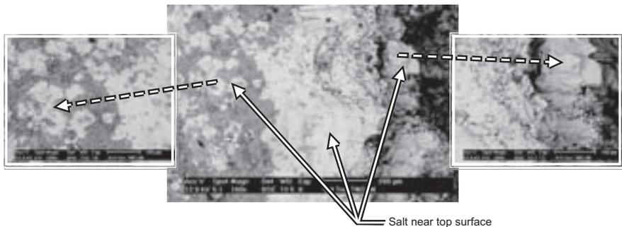
Figure 11: Halite efflorescence on the home made TNO plaster as seen by electron microscopy, showing at least three different crystal habits of the salt.
