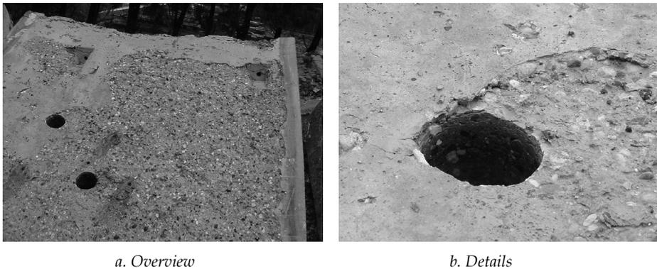
Figure 1: Portion of one of the tested concrete elements after the fire test showing some of the locations where the cores were removed for further analysis and damage due to spalling
