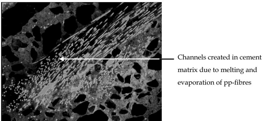
Figure 6: PFM-microphotograph taken at about 20 mm from spalled surface element, B, containing 3 kg.m<sup>-2</sup> pp-fibres. View is 2.7 mm x 1.8 mm.
