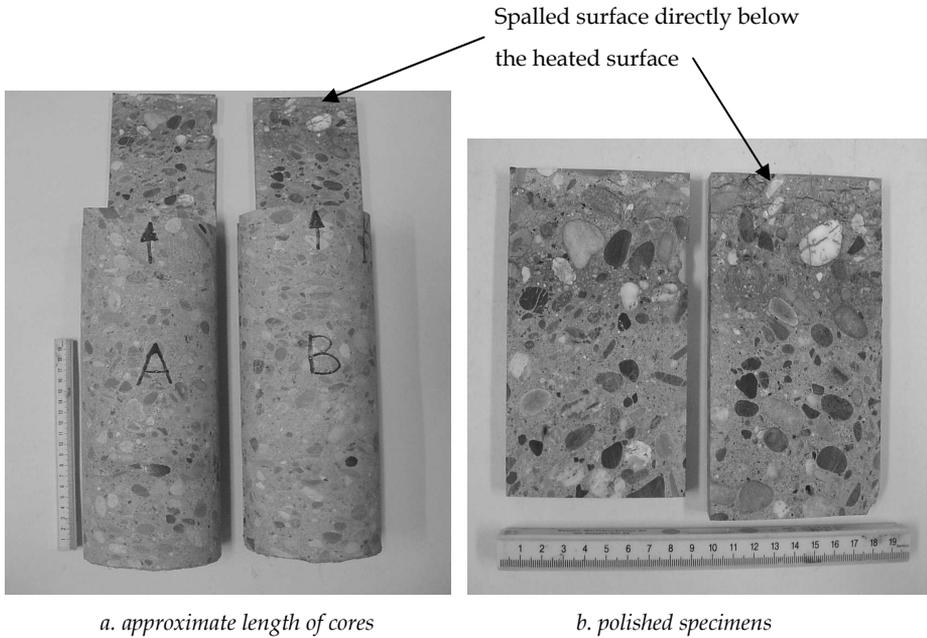
Figure 3: Overview of two cores showing areas where specimens were removed for further microscopic studies
