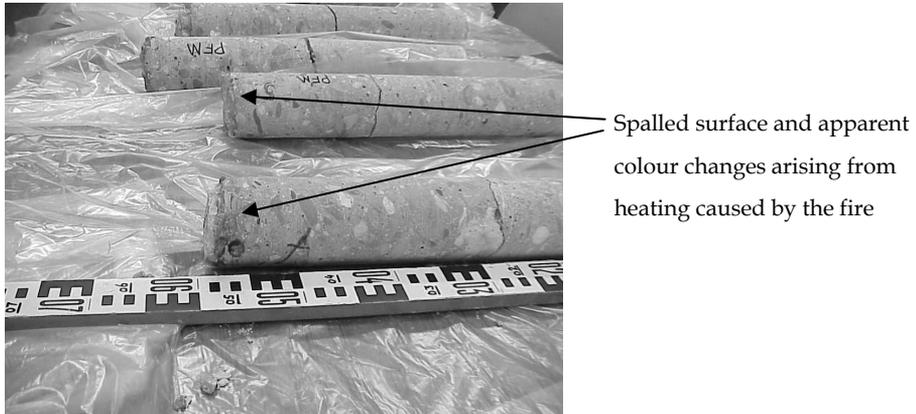
Figure 2: Overview of some of the cores removed from the two concrete elements for the microscopic studies showing the spalled surfaces and colour changes caused by fire heating
