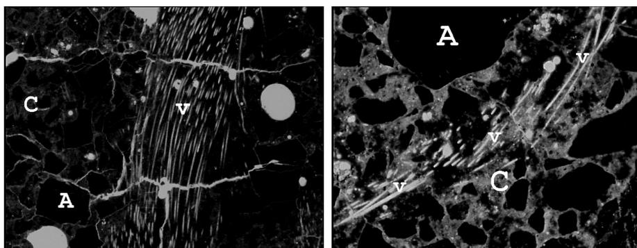
*a. element A, containing 1 kg.m<sup>-2</sup> pp-fibres*
