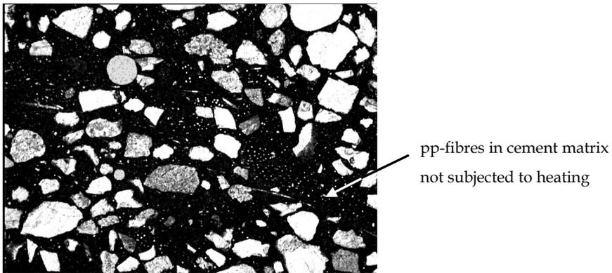
Figure 5: PFM-microphotograph of reference element, R2, containing 2 kg.m<sup>-2</sup> pp-fibres showing distribution of pp-fibres in cement paste matrix. Concrete was not exposed to fire. View is 2.7 mm x 1.8 mm.
