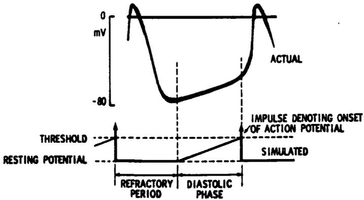
Figure 3. Schematic representation of an "integral pulse frequency modulator"
