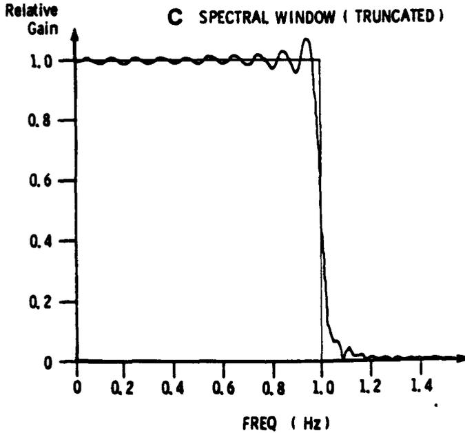
**Figure 6.** Logarithmic plot of the digital filter (0.5 Hz cut-off) when the weighting function is truncated to five cycles
