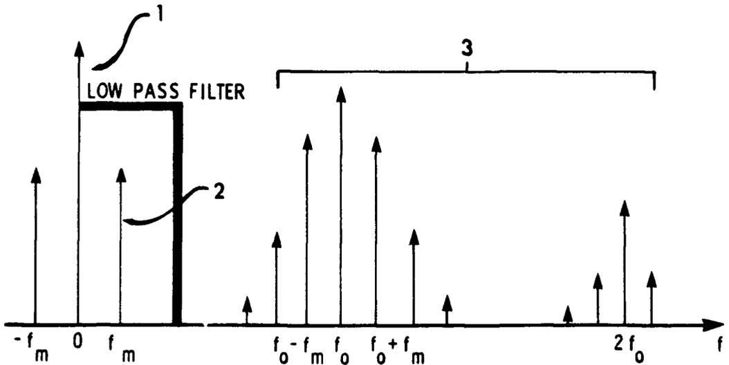
**Figure 5a.** The desired frequency profile of the digital filter
