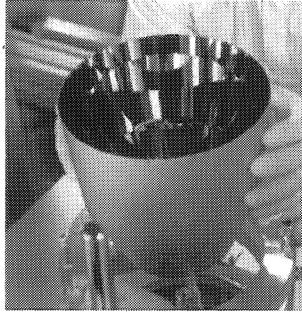
Figure 11. Individual shell for a grazing incidence collector.
