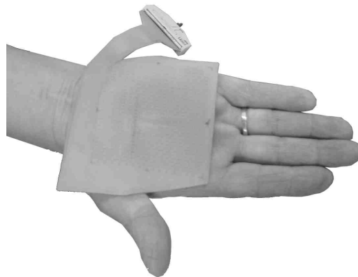
Figure 7.4 The hand mat was attached to the hand using double-sided adhesive tape
