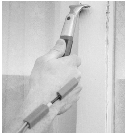
Figure 2.9 Example of wrist posture measurement, using goniometers.
