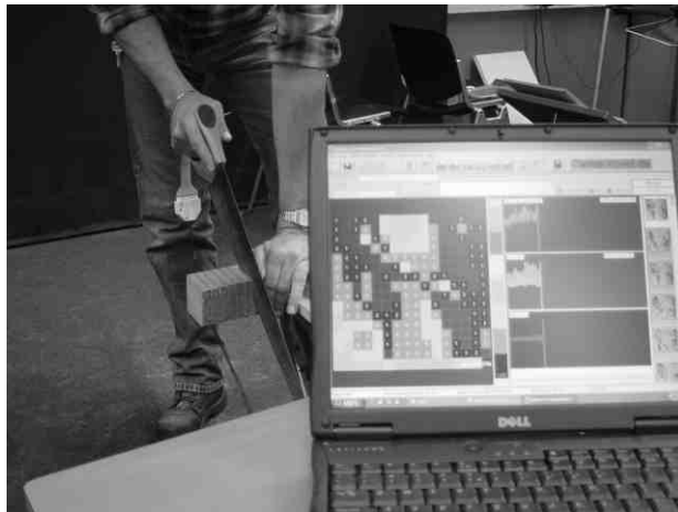
Figure 7.3 Dynamic contact pressure measurement
