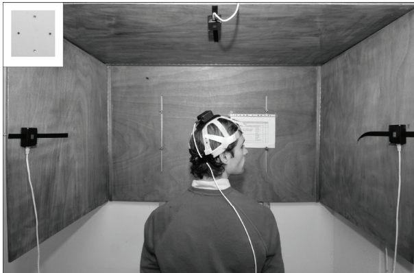
Figure 4.2: Experimental set-up for the head movement test. The cue display, positioned in front of the subject, is shown in the upper left inset. This display indicated the direction of the required head movement. Three target displays are visible; the fourth was positioned below and in front of the subject. The subject wore a movement registration device to measure head position and velocity.
