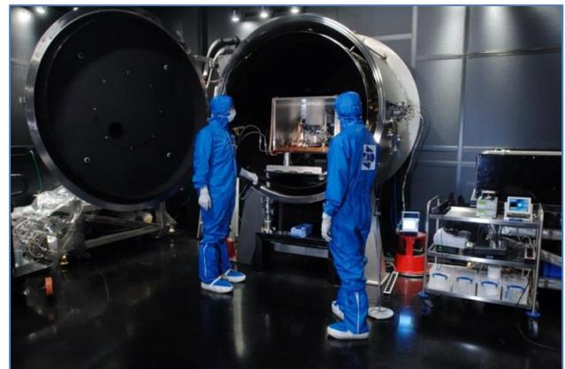
Figure 12: Thermal testing of BAM PFM: bar 2 on Invar set-up (left) and BAM in TNO VCF Thermal Vacuum chamber (right). Credits: TNO/Fred Kamphues
