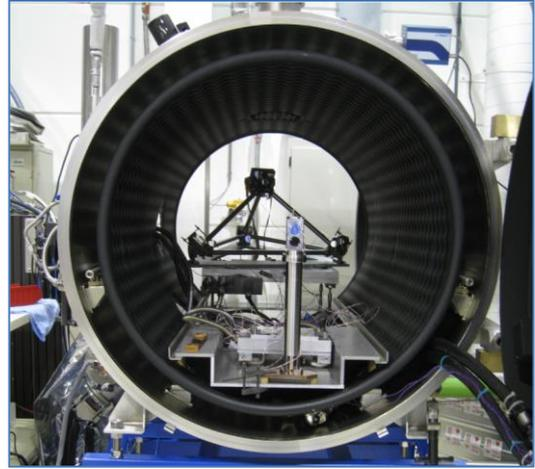
Figure 13: Stand-alone cryogenic test on Invar set-up: Left: Invar set-up with thermally de-coupled adjustable mirrors (7x). Right: Set-up in Thermal Vacuum chamber (right). Credits: TNO/Teun van den Dool.
