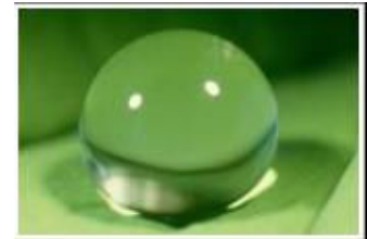
Water droplet on Lotus coating
