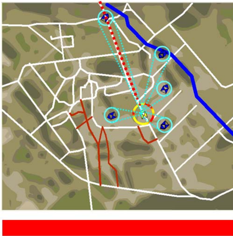
Figure 7. Computation of fratricide probability for all directions. In the shooting direction, indicated by the red dashed line, the probability of fratricide is high due to presence of a soldier in the line-of-sight.
