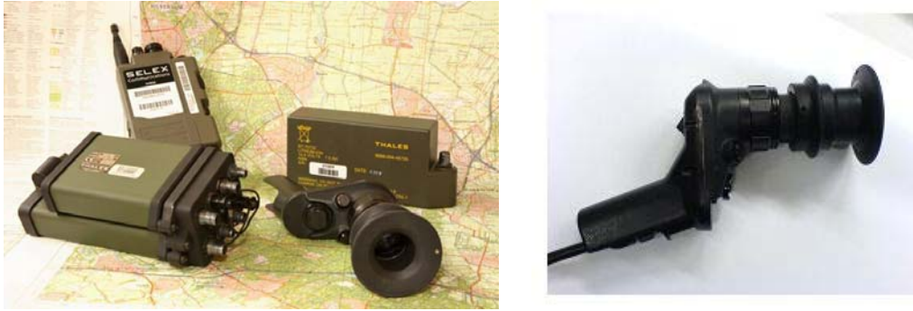
Figure 4. On the left, the hardware equipment CIM providing the situational awareness. On the right, a detailed image of the SMMI, a convenient interface of CIM.
