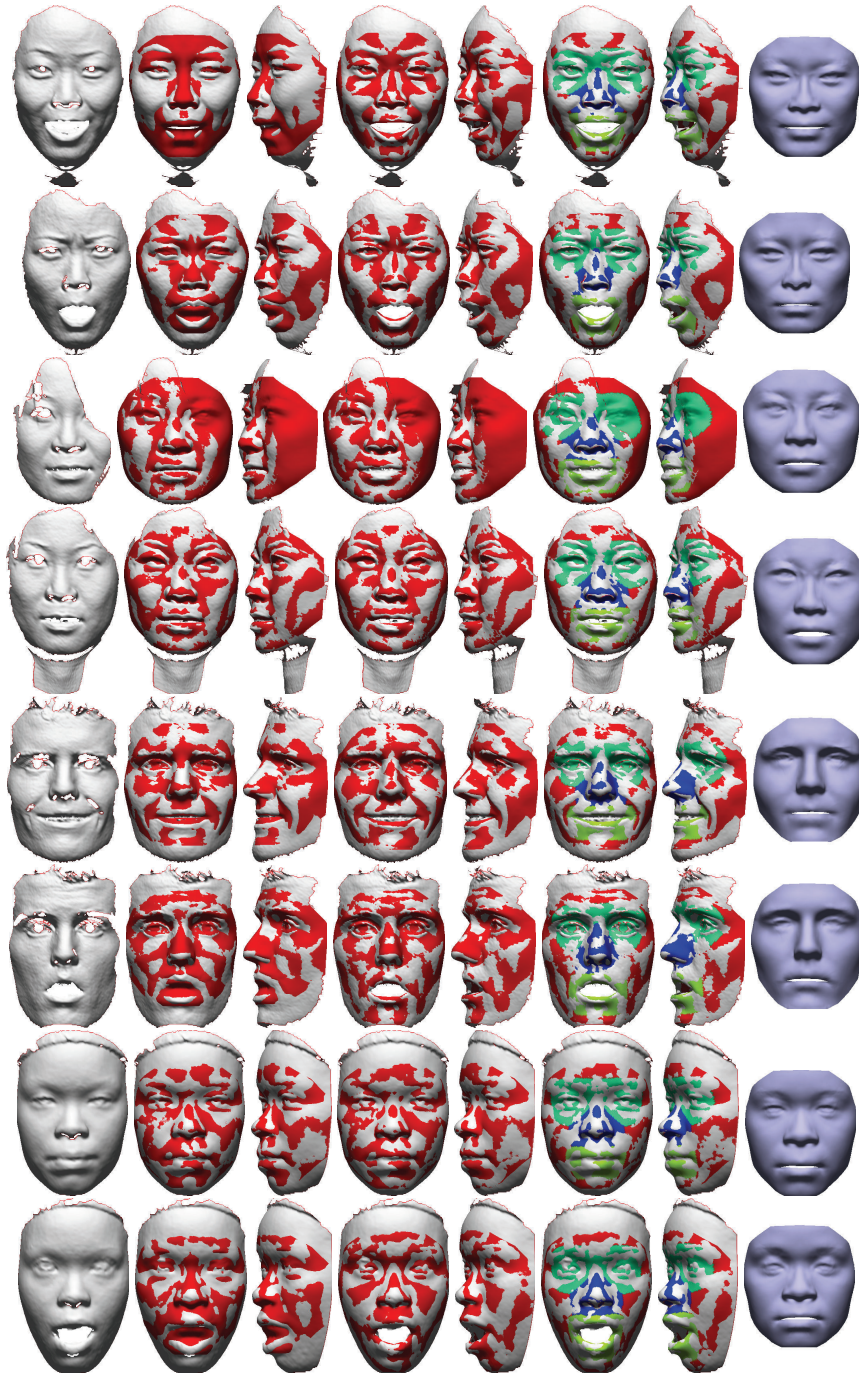
Figure 7.9: Model fitting to processed scans (1st column) using the neutral model only (2nd and 3rd column), a single component (4th and 5th column) and multiple components (6st and 7th column). The last column shows the neutralized face instances S_{expr.inst} - S_{expr} of the 6st column.
