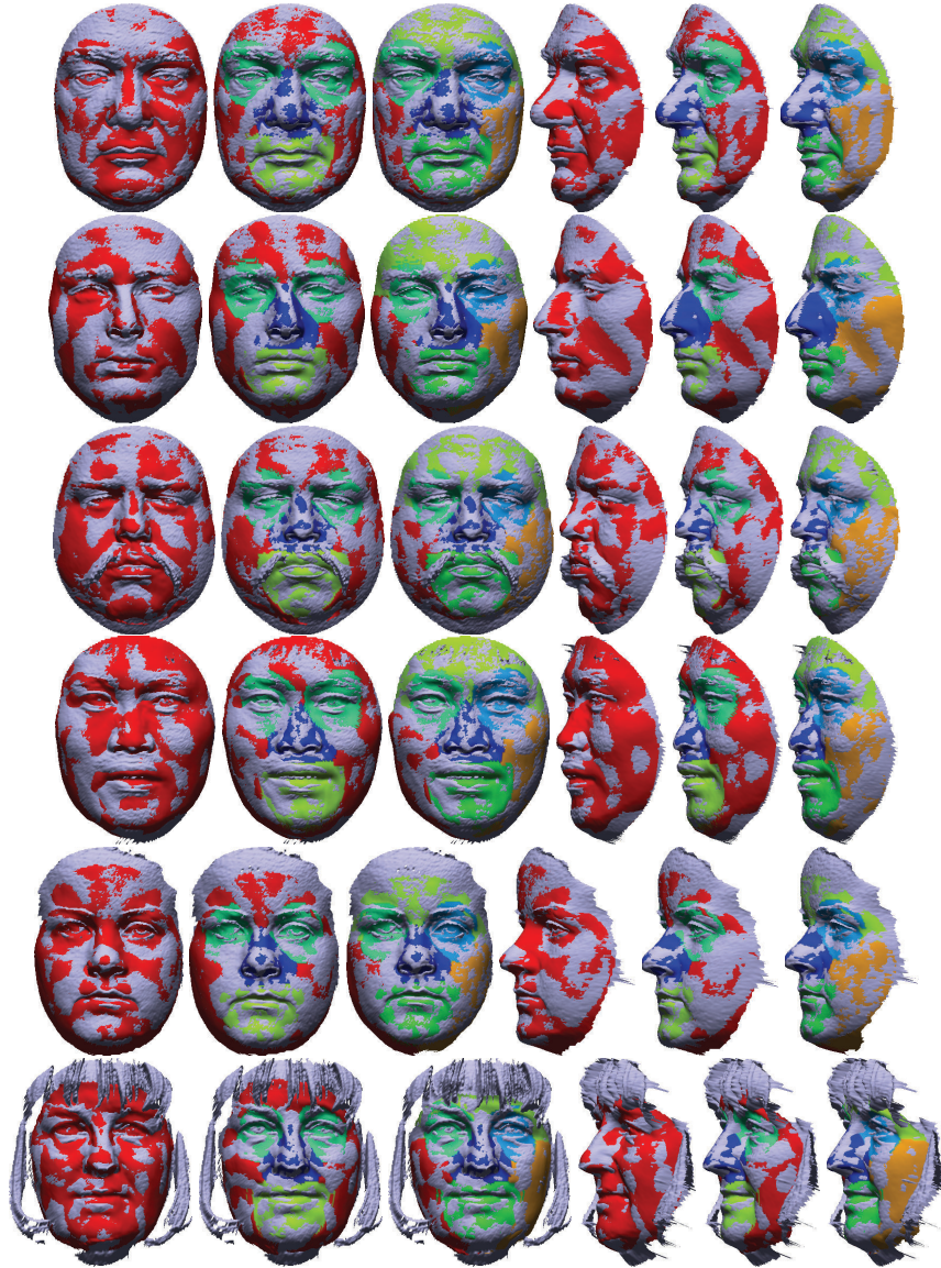
Figure 5.5: Fitted face models S_{final} based on a single component (1st and 3rd column) and multiple components (2nd and 4th column) to scan data in blue. Results from the front and side view, show a qualitative better fit of the multiple components to the scan data. The last two subjects on the right were also used in [18].
