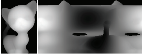
Figure 1.3: A depth image or range scan acquired from a plane scan (left) and a rotation scan (right).
