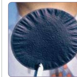
cnt based bucky paper for future bulletproof helmet
