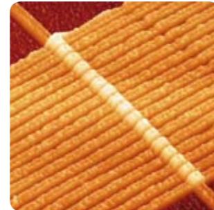
memory resistor structure at nanoscale
