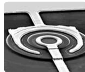
single photon source with quantum dots
