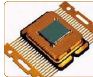
2D nanosized bolometer array for THz imaging (CEA-Leti)
