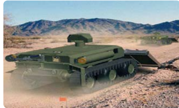
mine-detector ground penetrating radar Ho Missouri BAE
