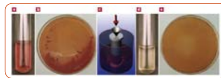
filtration of e-coli polluted water with CNT-filter
