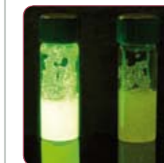
luminescent explosives detecting polymers (Fido)
