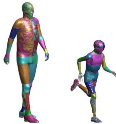
Figure 2. THUMS FE pedestrian models: 50 th male in walking position and 6 year old child in running position
