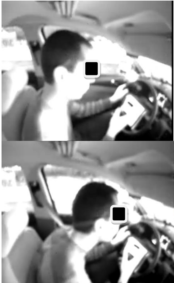
Figure 2. Occupant kinematics in Distracted-Automatic braking scenario, before braking (top) and at time of highest head excursion (bottom).
