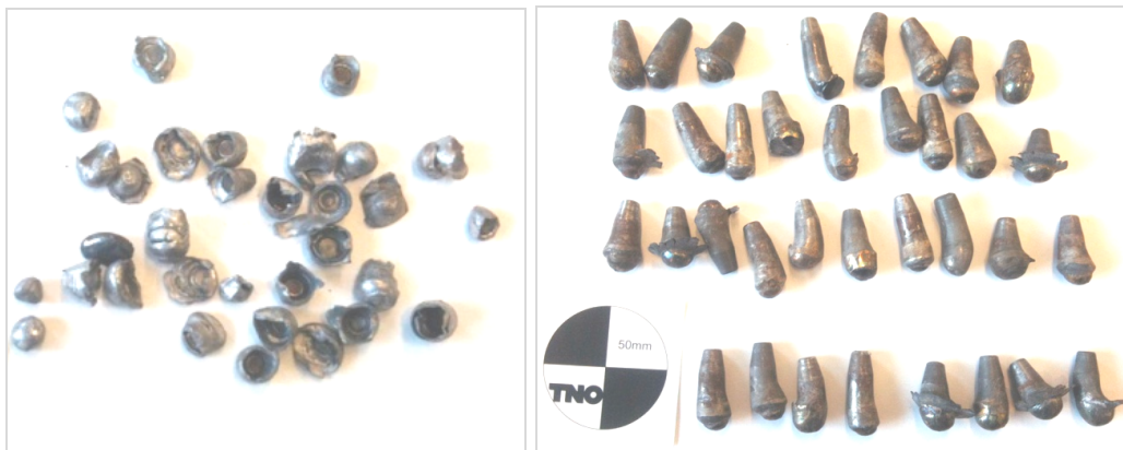
Figure 3: Deformed 7.62 Ball (left) and 0.50 Ball projectiles (right) after impact on steel targets
