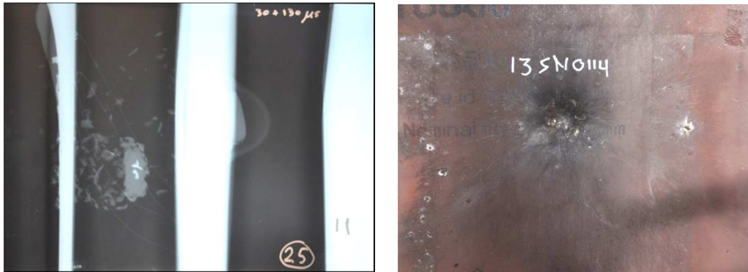
Figure 7 Denting of the RUUKKI Ramor 500 plate
