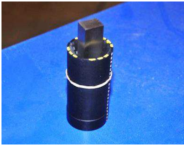
Figure 8 Bar projectile in composite sabot
