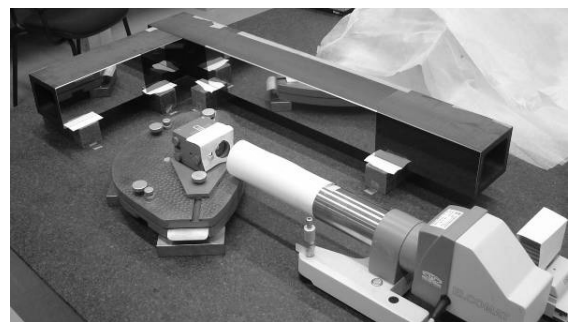
FIGURE 6: Silicon Carbide metrology frame during alignment
