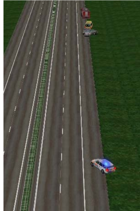
Figure 1: Birds-eye view of the simulation showing the directive “Flashing lights off on location”. The fend-off car signals (blue) flashing lights, the emergency vehicles have their flashing lights turned off.
