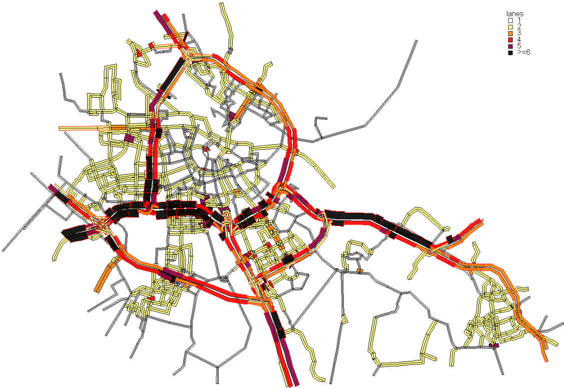
Figure 8.17: Total number of lanes after optimizing spare capacity
