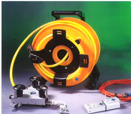
Cable reel, junction box and PDA transducer.
