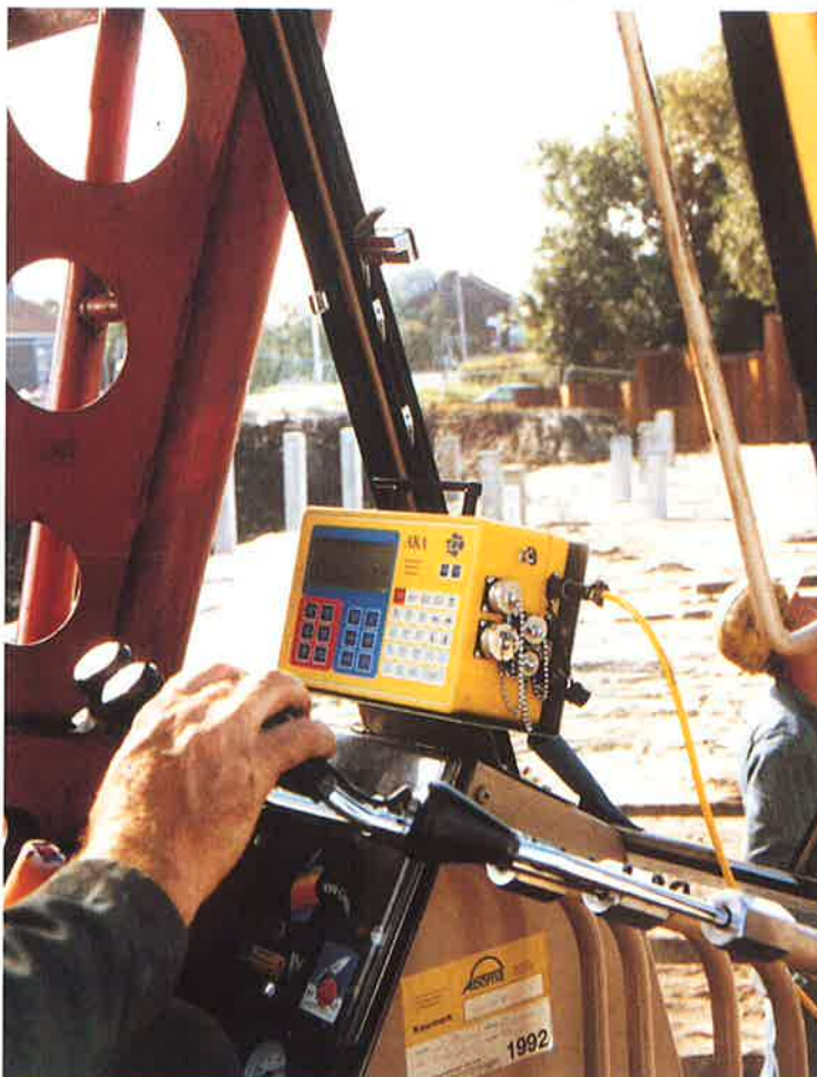
PDC microcomputer (FPDS- \alpha ) installed in a rig.
