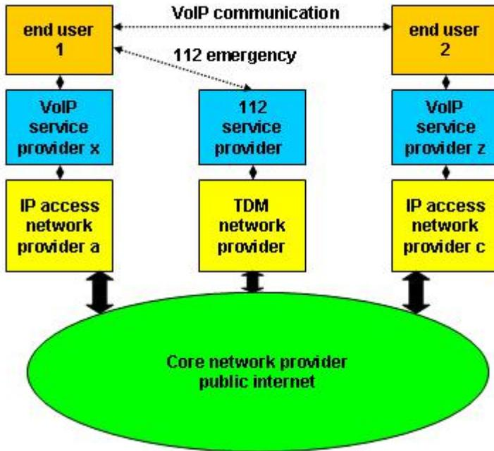
Figure 4: Illustration of the basic agreement for service interoperability for VoIP
