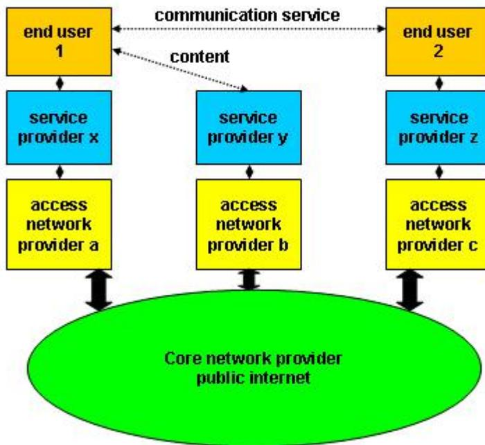
**Figure 2: broadband service interoperability at the level of service provider and access network provider**
