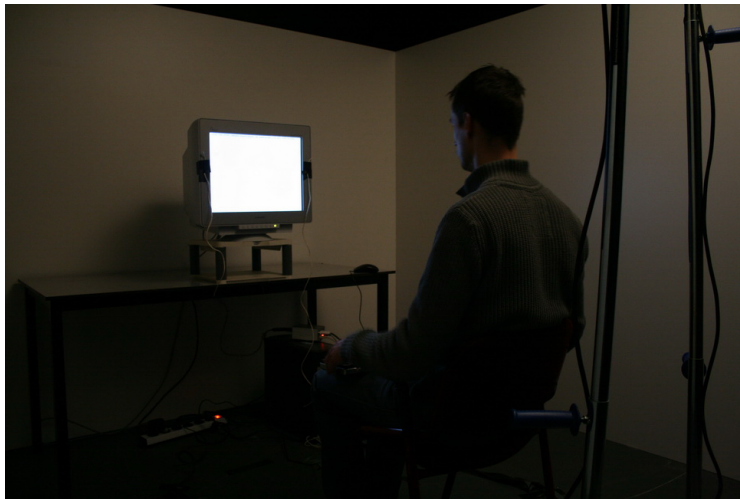
Figure 4 Experimental setup with observer at 106 cm from the screen.
