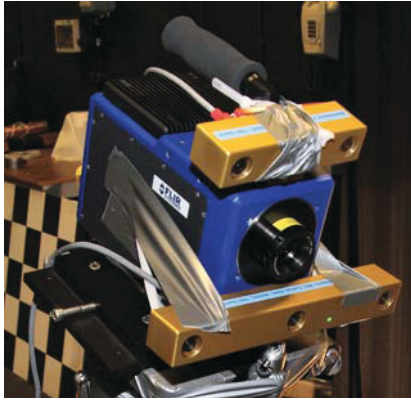
Figure 11. FLIR Titanium 560M IR camera (blue) with two stereo cameras (yellow). The bottom camera is the Point Grey Bumblebee XB3 stereo camera.
