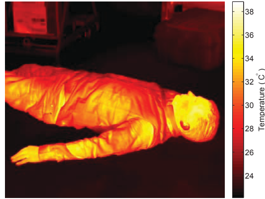
Figure 12. IR camera image with temperature indicated in pseudo colors. An absolute scale in degrees Celsius is given as a color bar on the right side.
