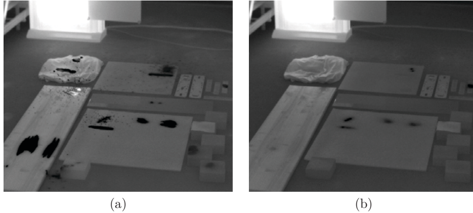
Figure 10. IR images with traces of sperm, water and blood with water on different materials. (a) - right after putting the sperm on to the material; (b) - 5.5 hours later.
