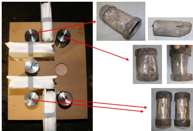
Figure 2 Test at TNO with mitigating materials placed between donor and acceptor shells [2].
