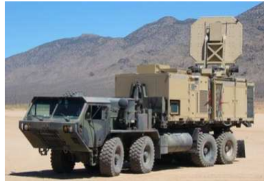
Figure 3. High Power Microwave mounted on a 8 wheeled truck.
