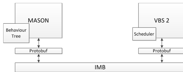
Figure 23. Overview of the implementation of MASON and VBS2 and the connection.
